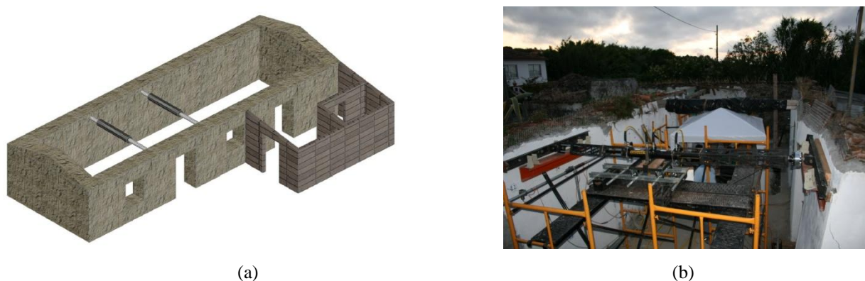
Fig. 9: Experimental test setup used in test #2 and test #3: (a) schematic representation of setup; and (b) in situ implementation for tests (interior view) (A. A. Costa, Arêde, Costa, & Oliveira, 2011)
