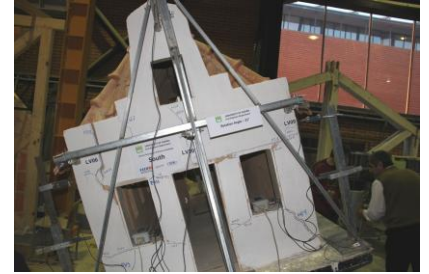
Tilting table test of a reduced scale model of a typical adobe house from Aveiro performed at the University of Aveiro
